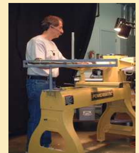
Turning with a laser arm that shoots a point onto the wood
