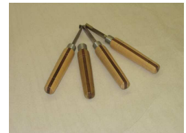
Ernest Lowry Thread Tools - Maple/ Walnut Handles Briwax Sanding Sealer/ Briwax Polish & Briwax Polish
